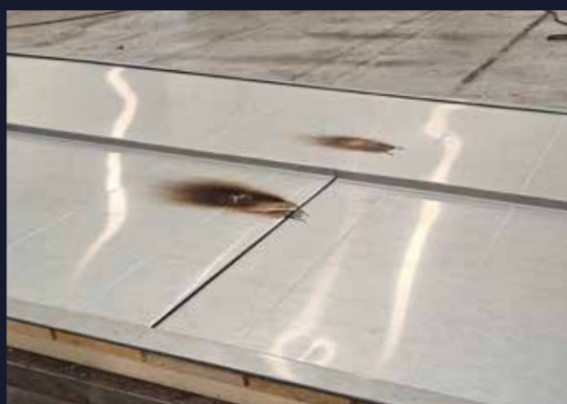
A sample of the system after the test, with the titanium-zinc zintek® surface still intact
